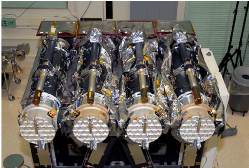
Figure 2.2: The instrument package of AIA consists of four telescopes, each of which has its own guiding telescope mounted on top. The instrument has been assembled in a clean room at NASA Goddard Space Flight Center before being mounted on the SDO spacecraft (see Fig. 1 in Lemen et al., 2012 ).
