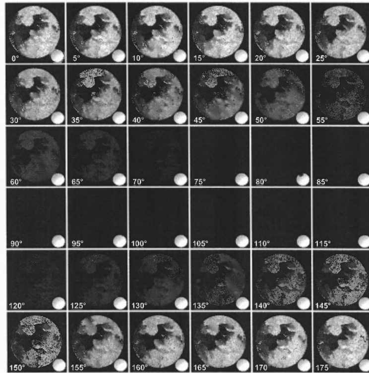
Figure 7.15 Average intensity as a function of the rotation angle of the second linear polarizer.
