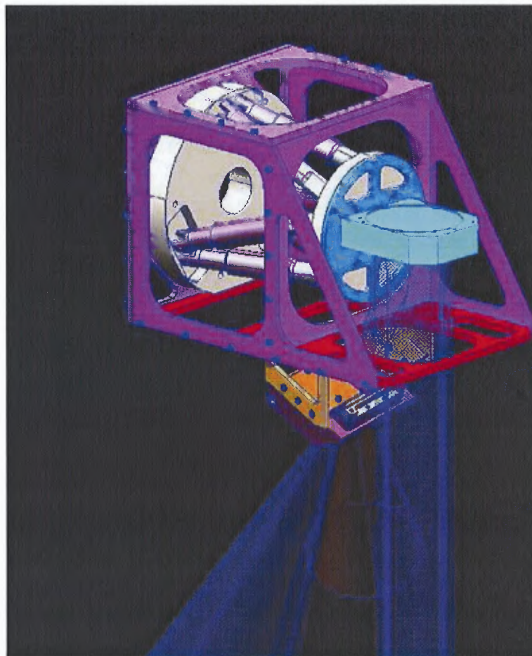
Figure 3.5 CAD rendering of the M2 mirror mounted on the Physik Instrumente M-850 hexapod system (light gray) with the heat stop in place (courtesy of Jeff Kuhn).
